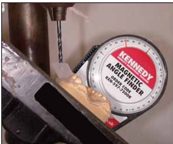
Fig. 7 Working cast mounted on adjustable table at 45° angle to vertical plane, as indicated by magnetic angle finder, for channeling through acrylic block with 4mm drill press.
