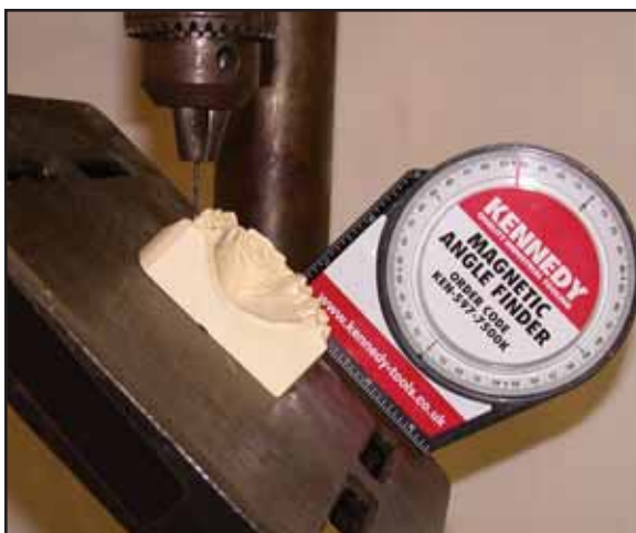
Fig. 3 Working cast mounted on adjustable table at 45° angle to vertical plane, as indicated by magnetic angle finder, for drilling.
